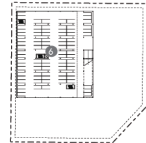
proposed underground parking typical 80 parking spaces | 33,800sf/floor
